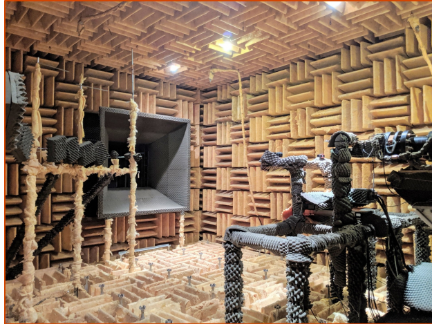
Fig. 6 Anechoic Chamber at Skytop Turbulence Laboratories, Syracuse NY.
