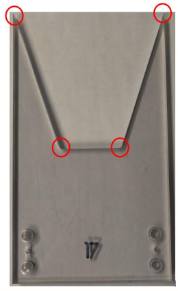
Fig. 11. Example Aft Deck Plate With Highlighted Coordinate Points
