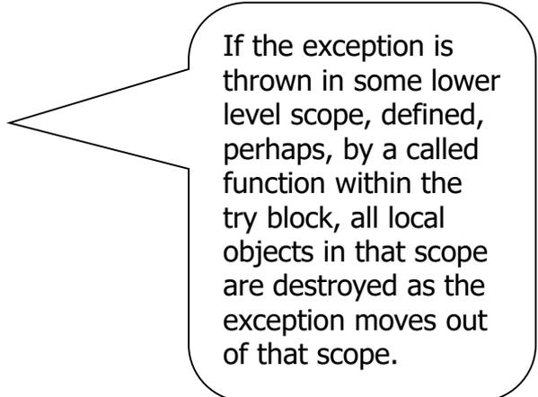
If the exception is thrown in some lower level scope, defined, perhaps, by a called function within the try block, all local objects in that scope are destroyed as the exception moves out of that scope.
