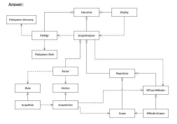
ScopeAnalyzer owns a configParser object, not shown for lack of space, that owns the Parser, Repository, and all Rules and Actions. It gets a file specification from FileMgr and uses Parser to analyze its code scopes. The ScopeAction stores the Scopes in MTree. At the end of analysis ScopeAnalysis returns to Executive which then calls Display to display the required scope information and one tree's XML. XmlWriter has also been elided for lack of space.
