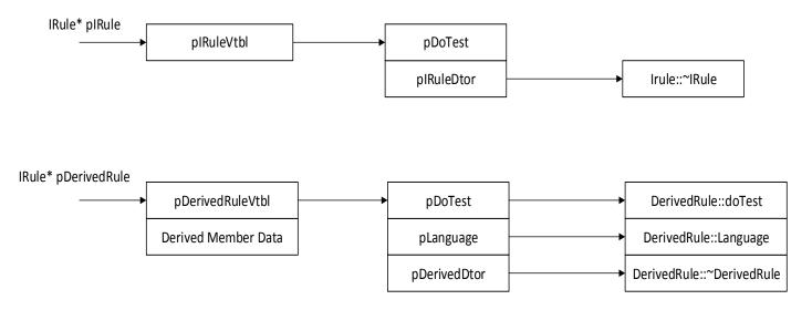
IRule::addAction and IRule::doActions are not virtual and so do not have entries in the IRule vtbl. IRule::doTest is pure virtual so it has an entry but no corresponding implementation.
