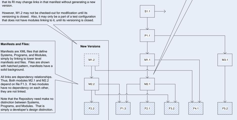
Manifests are XML files that define Systems, Programs, and Modules, simply by linking to lower level manifests and files. Files are shown with hatched pattern, manifests have a solid background.
