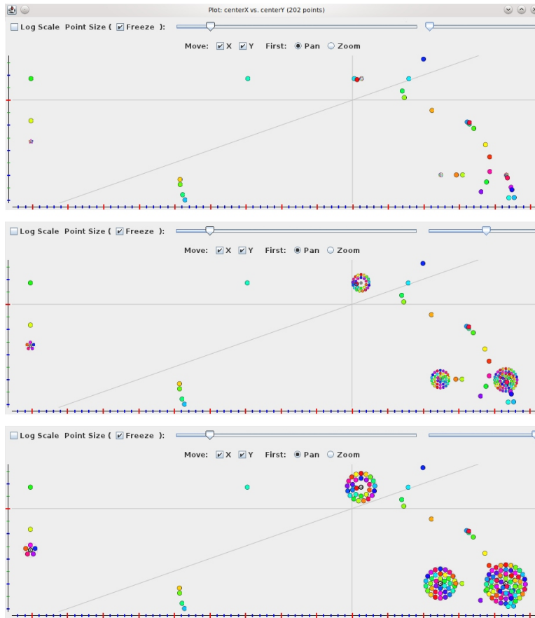
Figure 4.13: A VERDICTS X-Y Plot shows relationship between any two traced (possibly user-defined) variables. The plot above is for variables centerX and centerY. Repeated values of (x,y) across calls can be expanded into packed circles as seen in these plots. Clicking on a circle opens up the Method Call View for that call.
