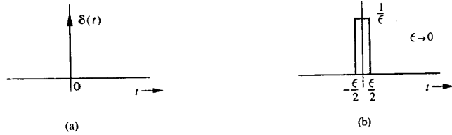
Fig. 1.19 A unit impulse and its approximation.
