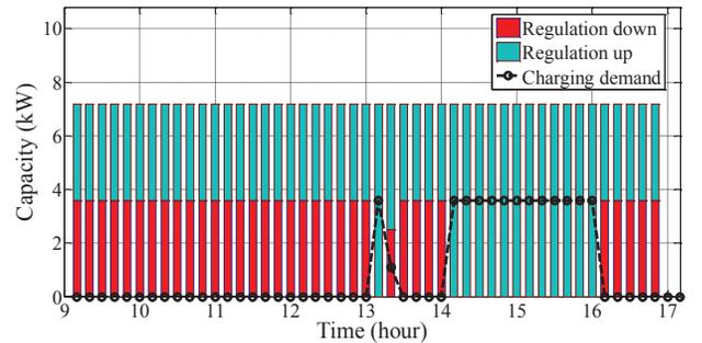
Fig. 2. Optimal charging demand and offered regulation capacity of the EV.
