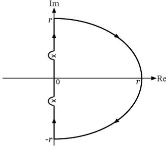
Fig. 2. Closed contour  $\mathfrak{D}$  traversed in the clockwise direction taken as the Nyquist path as  $r \rightarrow \infty$ . The indentations are made to avoid the eigenvalues of  $\mathcal{A}$  (i.e., open-loop modes) on the imaginary axis.
