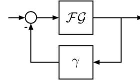
Fig. 1. Closed-loop system  $\mathbf{S}^{\text{cl}}$  in the standard form for Nyquist stability analysis.
